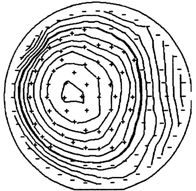
Figure 15. Four-Point Probe Contour Map After a Furnace Phosphorus Pre-Deposition
